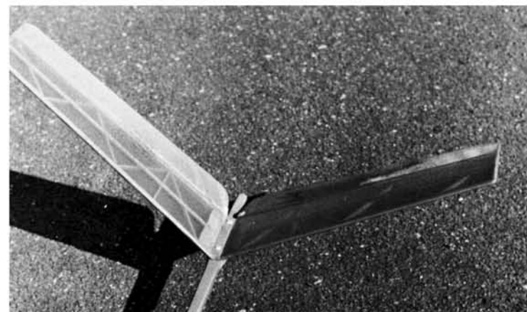
The "V" tail, easily built, nice in that it is graceful, high above ground on the landing roll. Popular on full scale soarers for this reason. Linkage can be seen on photo to right. Two horns are required. Bottom right photo captures the winch mechanism, foot treadle etc. Or use a hi-start line deal. Beneath: The nose, no room lost for a thin cross-section. It balances well.
